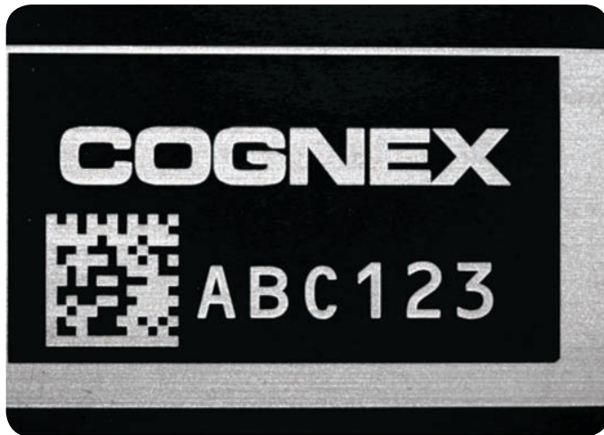
Figure 9a: Image taken of a moving part using strobe light illumination.
