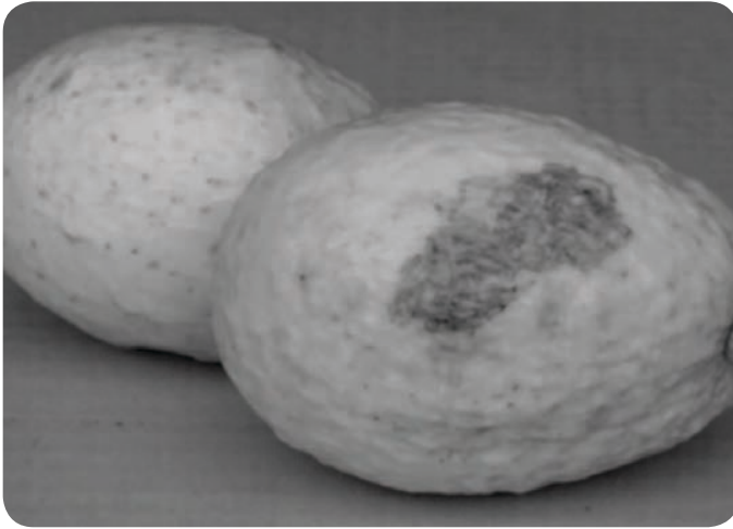
Figure 2: Infrared light through a filter highlights bruises on fruit.
