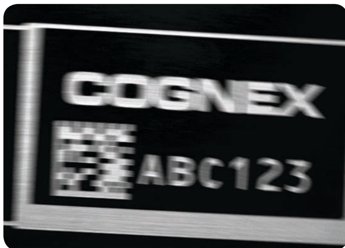
Figure 9b: Image taken of a moving part using continuous illumination.
